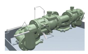
2. Lift the clapper system of the valve, remove debris.
