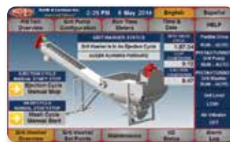
Grit Washer Overview
