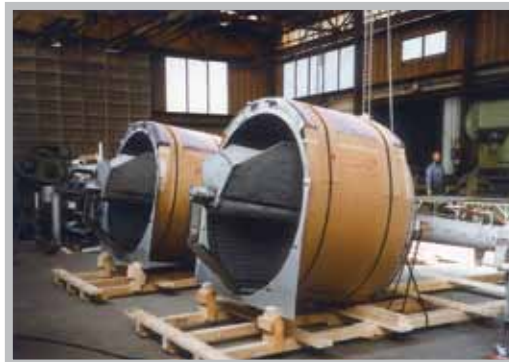
Pictured at left: Two large diameter SCHLOSS™ Mark XV-C™ fine screw screens are being prepared for shipment following fabrication at the S&L Schloss™ U.S. fabrication facility.
